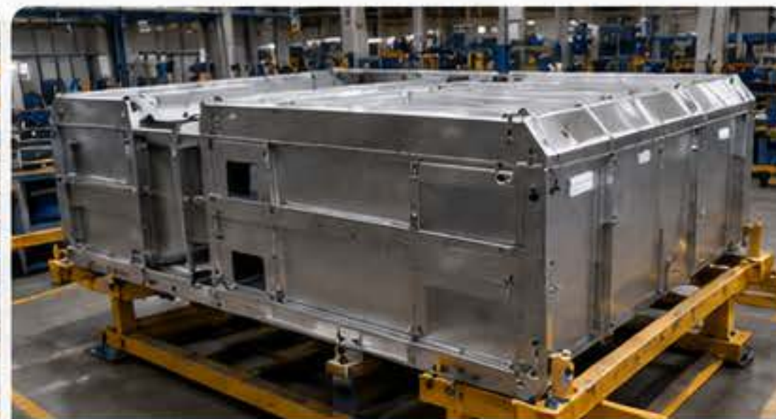
BATTERY ENCLOSURE MANUFACTURING
