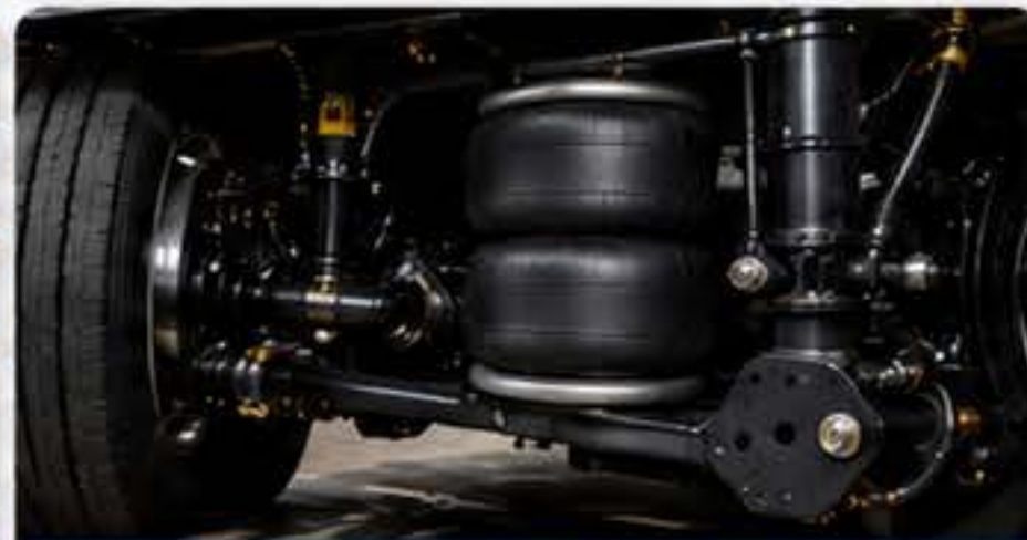
AIR SUSPENSION DETAIL
